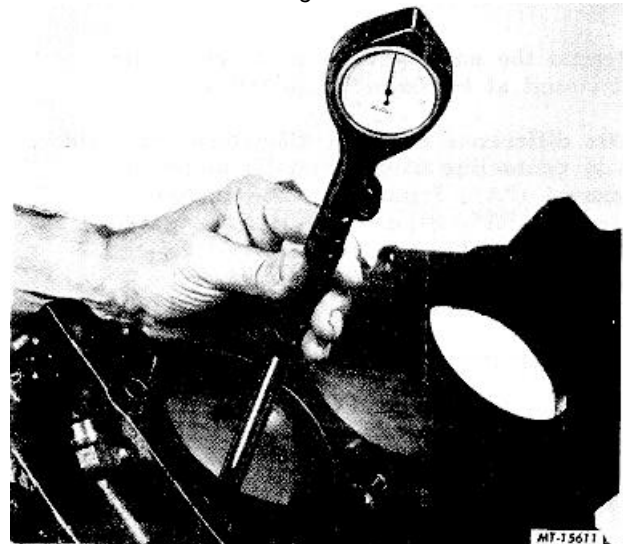
Fig. 88 Checking Cylinder Bore with Dial Bore Gauge
