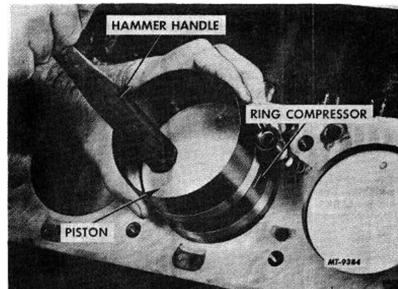
Fig. 149 Installation of Piston in Cylinder Block
