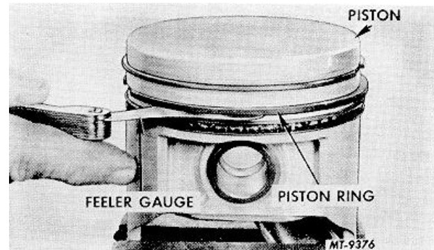
Fig. 85 Checking Ring-to-Groove Side Clearance with Feeler Gauge
