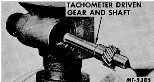
Fig. 33 Removing Tachometer Driven Gear And Shaft
