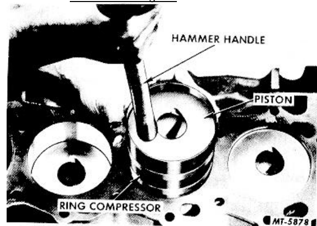
Fig. 158 Installing Piston and Connecting Rod Assembly
