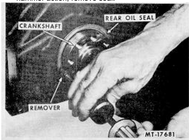
Fig. 63 Removing Rear Main Bearing Cap Oil Seal from Installed Crankshaft
