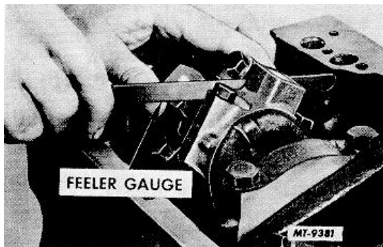
Figure 123 Checking Connecting Rod End Clearance
