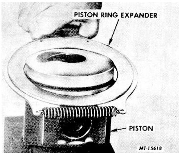
Fig. 84 Installing Piston Ring Using SE-1149 Piston Ring Expander Tool
