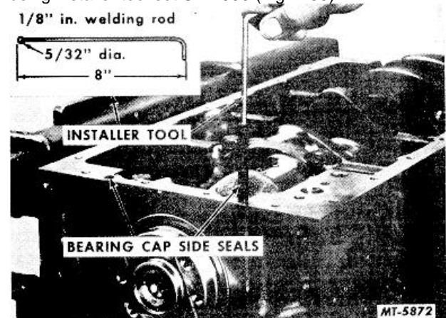
Fig. 154 Installing Rear Main Bearing Cap Side Oil Seals
